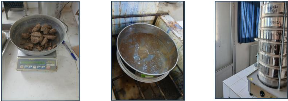
Figure 3.2. Particle size analysis test by wet sieving.
